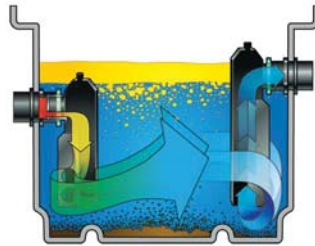
Trapper II™ Side View with Diffusion Flow™
